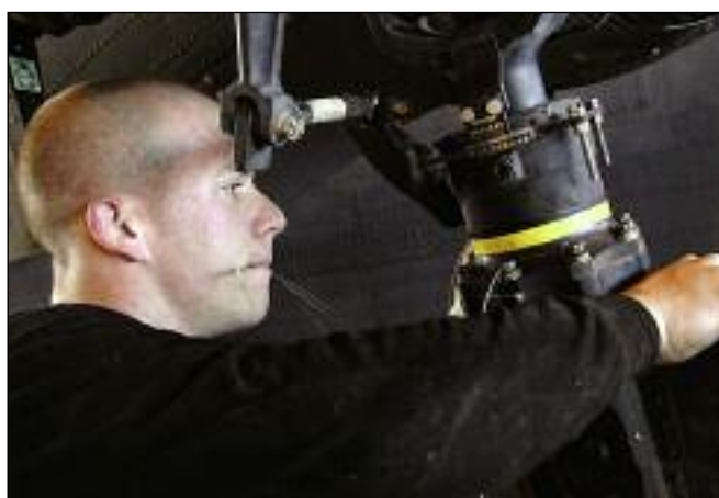
▶ Airman 1st Class Matthew Holliman threads safety wire while helping to reassemble the MH-53.
